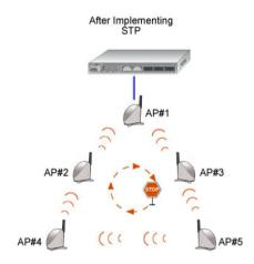
Spanning-Tree Protocol operation is transparent to end stations, which are unaware whether they are connected to a single LAN segment or a switched LAN of multiple segments.
