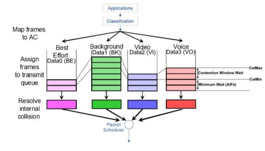
The following steps demonstrate how to configure these WMM Parameters.
