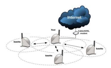
Here, the root gateway connects to the Internet and maintains three WDS links while each satellite gateway uses one port only for communication with the root.
