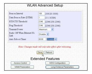
The **Beacon Interval** is the amount of time between beacon transmissions. A beacon is a guidance signal sent by the access point to announce its presence to other access points. It also sends information, such as timestamp, SSID, and other parameters regarding the access point to other access points that are within the specified range. The access point needs the beacon interval to know when to receive the beacon from the other access point.
