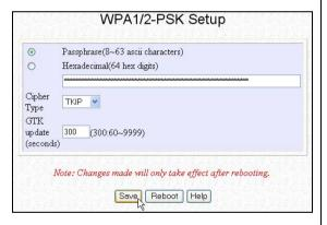
If you are using the **Passphrase** format, your entry can consist of a minimum of 8 alphanumeric characters or a maximum of 63 alphanumeric characters.
