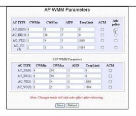
Depending on the mode you set up, you have to select either AP (Access Point) or BSS (Basic Service Set) WMM Parameters. For instance, if the mode is AP, select AP WMM Parameters. The following parameters are described:
