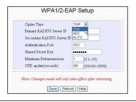
You can key in a different Authentication Port but it <u>MUST</u> match the corresponding port of the RADIUS server.
