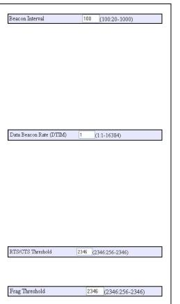
This value extends from 256 to 2346 bytes, where a value of 0 indicates that all the packets should be transmitted using RTS.
